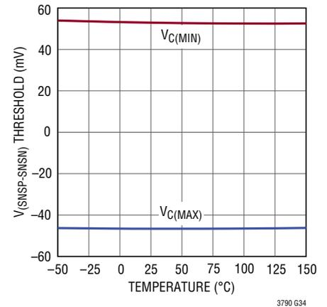
**$V_{(SNSP-SNSN)}$  Boost Threshold vs  $V_C$**
