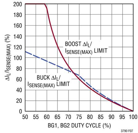
**Figure 7. Maximum Peak-to-Peak Ripple vs Duty Cycle**
