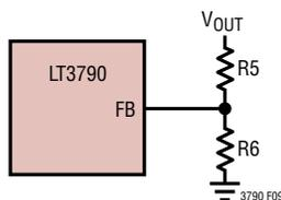
Figure 9. Resistor Connection for Constant Output Voltage Regulation
